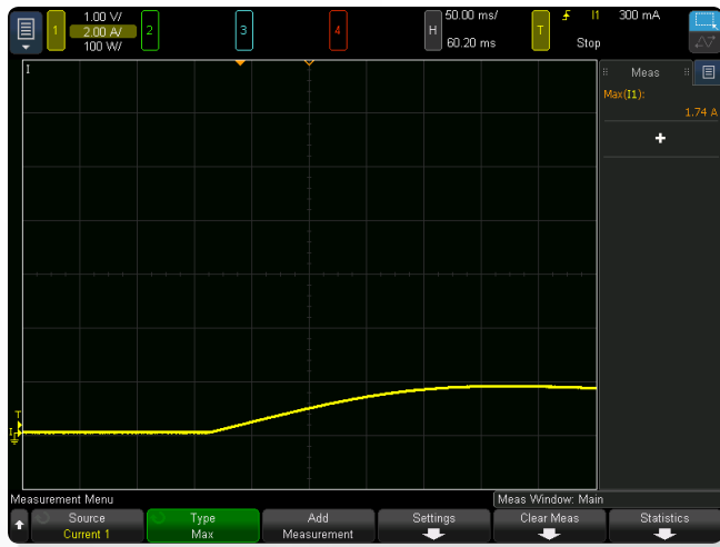
Figure 6. The variable slew rate of 10 V/s eliminates the inrush current
