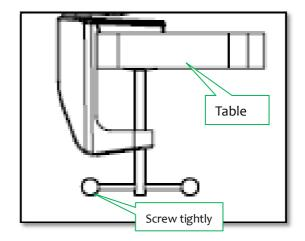
3. Insert the bottom stem of the **Folding Arm** into the **Clamp.**
