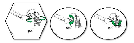
Note: Before turning the **Camera Head**, please set the **Tighten Knob** on both side of the Camera Head to ensure the head loose enough to operate.
