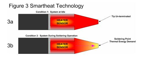
The net result is a soldering tool that directly controls the power to the solder pad by eliminating one source of thermal latency and dramatically reducing both the stored energy and tip geometry latency as is shown in Figure 3b. The benefit is reliable, repeatable direct process control.
