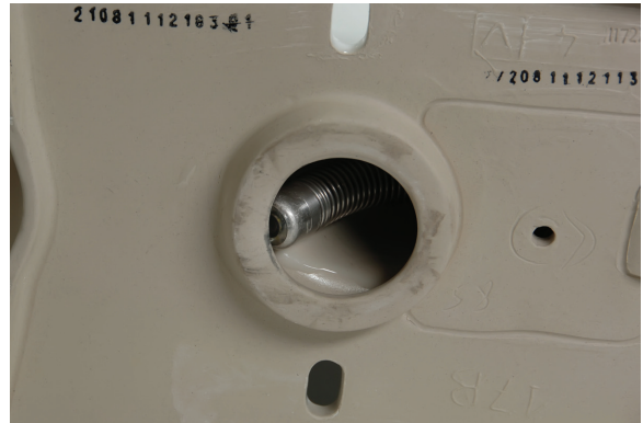
Figure 17 – Camera Head Blocked in Turn
