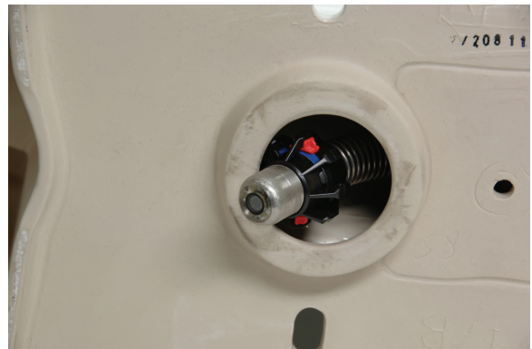
Figure 18 – Camera Head with Ball Guide in Turn
