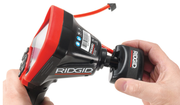
Figure 10 – Connecting the micro CA-300 Camera Monitor
