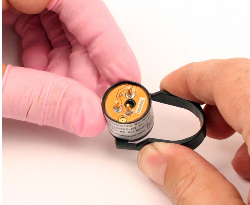
Figure 35: Using Removal Tool
