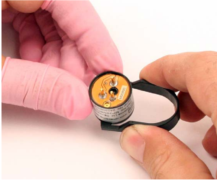
Figure 29: Using Removal Tool
