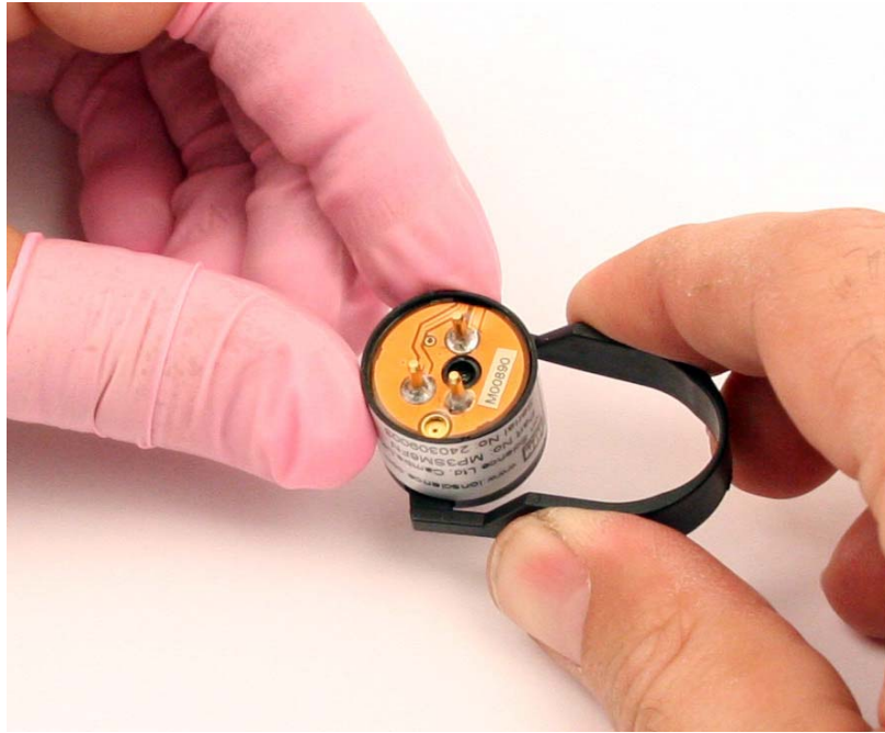
Figure 33: Using Removal Tool
