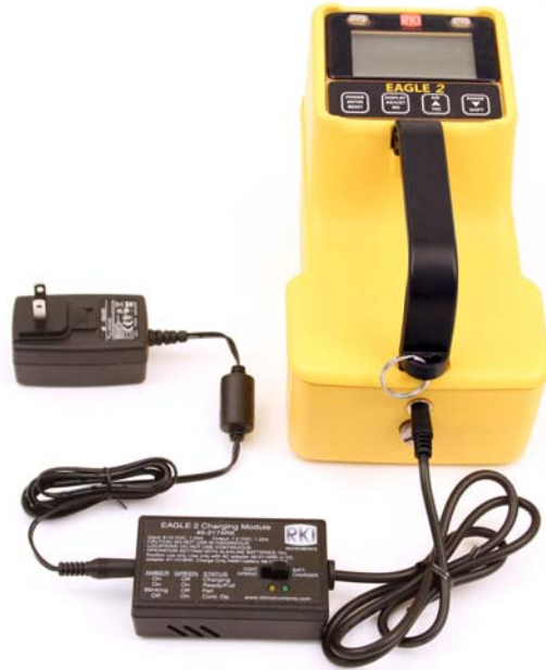
Figure 17: Connecting the EAGLE 2 to the Charger
