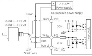
PLC DC input circuit
