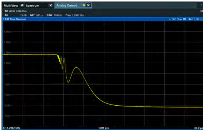
Frequency settling behavior of an oscillator
