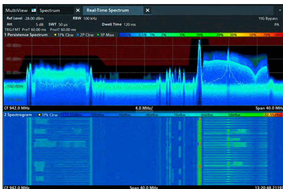
Real-time spectrum with frequency mask trigger in cellular band
