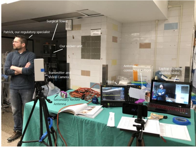
Figure 1: Indago's test setup for on-site measurements
