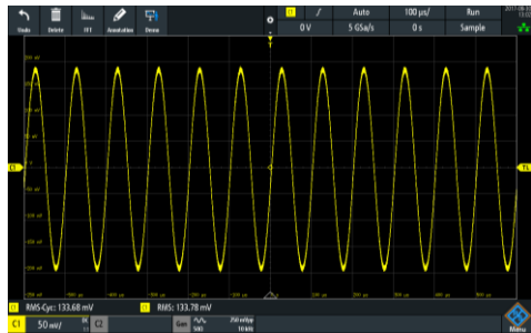
R&S®RTM3000: 10.1" display, 1280 x 800 pixel resolution
