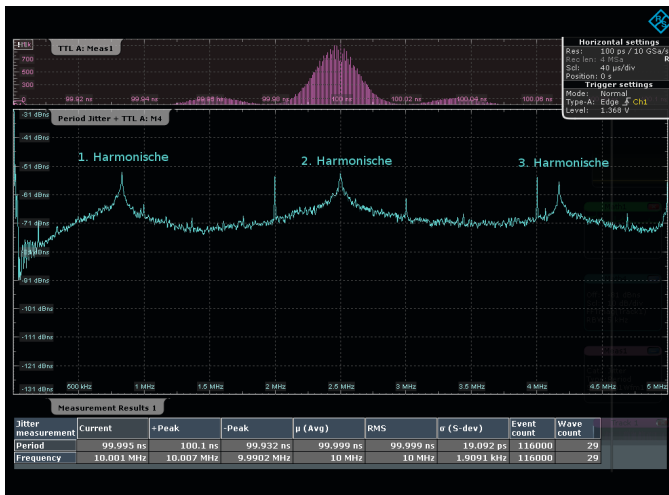
Track spectrum (cycle-cycle jitter) for identifying interference frequencies.
