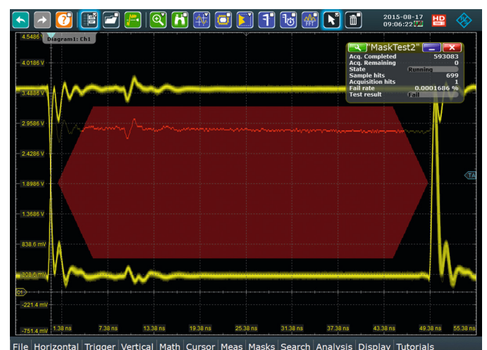
Fast mask test: Within ten seconds, more than six million waveforms are acquired, evaluated and displayed.
