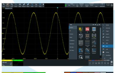
The signal bar displays fundamental parameters of activated signals. In addition, a signal preview is shown for minimized signals.
