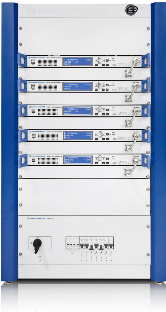
End-of-line test: rack with four operational R&S®SFE100 test transmitters and one spare unit
