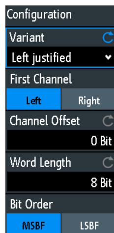
Figure 12-39: Setup menu Audio Left Justified Variant
