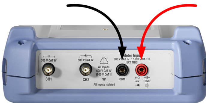
Figure 4-1: Meter inputs to connect test leads
