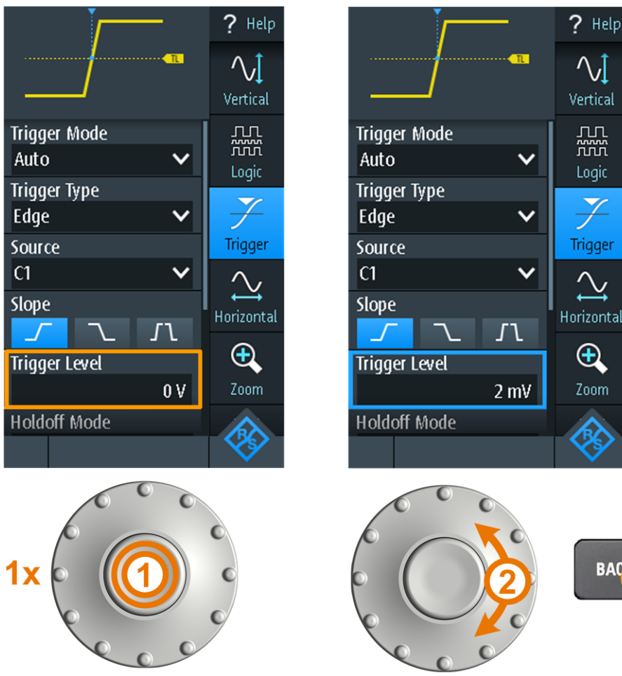
Figure 4-6: Set numerical value using the wheel
