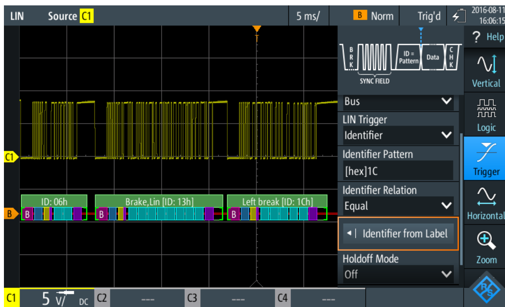
Figure 9-36: Trigger on identifier "Left brake"
