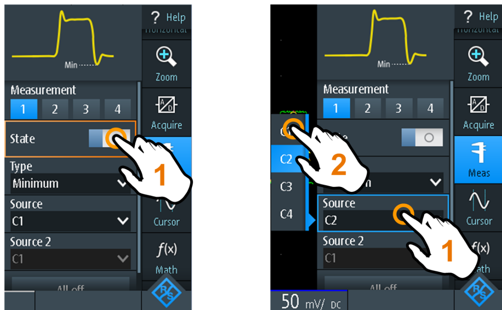
Figure 2-7: Switch on or off (left) and select a parameter value (right)
