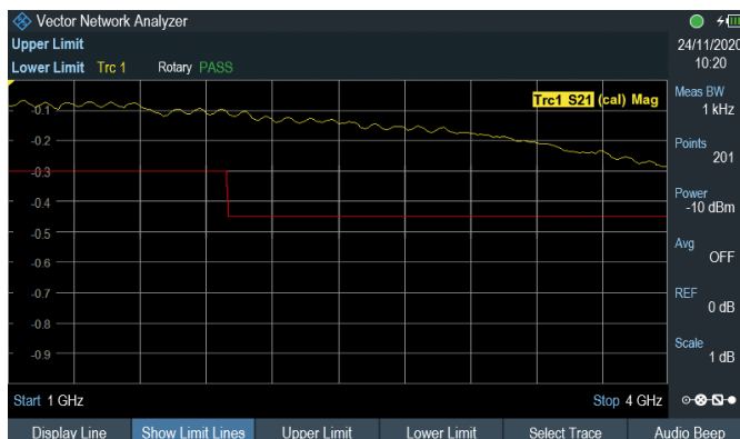
Fig. 2: S_{21} insertion loss measurement.
