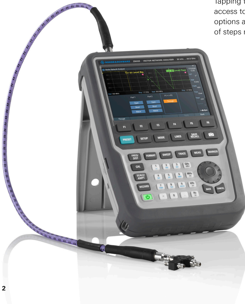
R&S®ZNH with flexible calibration approach - user-define sequence.
