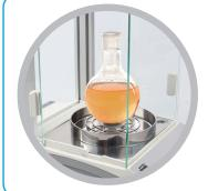
Enlarged Weighing Chamber and open-door clearance allow easy access to the weighing pan and facilitates use of laboratory glassware of various sizes and dimensions.
