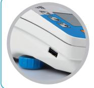
**Ease of Communication** with peripherals due to placing of the USB interface at the chamber front.
