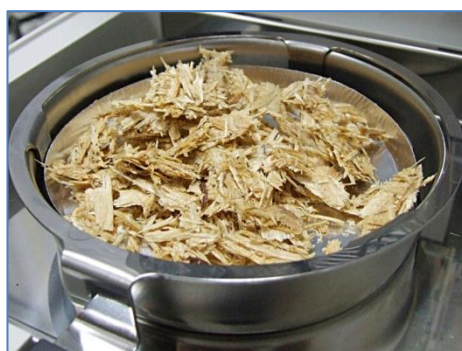
Photo 12. Chipboard – disintegrated sample (appropriately prepared material)
