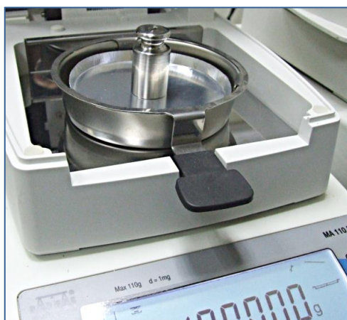
Photo 2 Adjustment of MA 110.R moisture analyzer (100 g mass standard)
