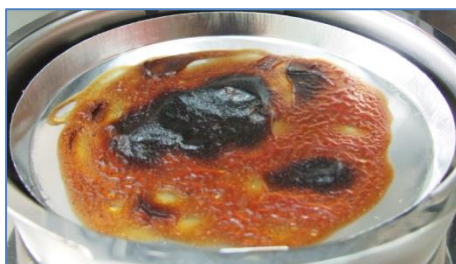
Photo 17. Crust formed on the sample's layer
