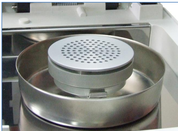
Photo 21. Tester placed inside the moisture analyzer
