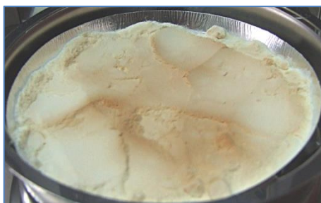
Photo 18. Surface burning – colour change
