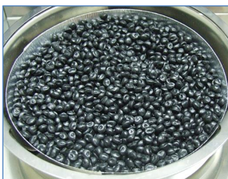
Photo 19. Samples of dark colour = higher drying temperature
