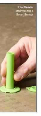
After the initial equilibration has been reached per ASTM F2170 requirements, subsequent readings can be taken instantly. If future testing is needed, replace the protective plug by pushing it back into the protective cap.
