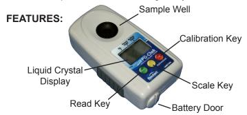
Using a PG-Chek to test freeze points following the American Society for Testing & Materials (ASTM) Standard Practice D3321 provides results that are precise to  $\pm 1.0^{\circ} F$  ( $\pm 0.6^{\circ} C$ ) reading a 50 vol % aqueous solution of propylene glycol. By comparison, a hydrometer is only precise to  $\pm 8.0^{\circ} F$  ( $\pm 4.4^{\circ} C$ ).
