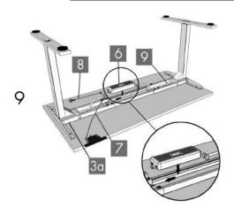
Slide the Control Box (part 6) onto the Frame End-CB (part 3a).
