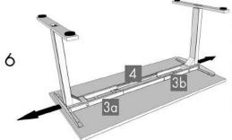
Your desktop may or may not be pre-drilled. Check both sides of the desktop before placing the desk base on the underside of the desktop.
