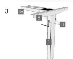
The Frame End-CB (part 3a) should be placed on the side of the desk where you plan to mount the Control Box (part 6) and the Handset (part 7).
