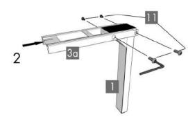
Place one of the Legs (part 1) into the Frame End-CB (part 3a) ensuring that the bar (arrow) is on "top" in relation to the Leg (part 1).
