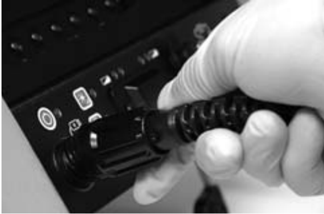
Figure 13 – Connecting To A SeeSnake CCU
