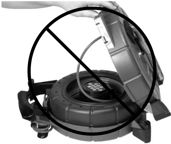
Figure 10 – Do Not Allow Cable to Uncoil Freely
