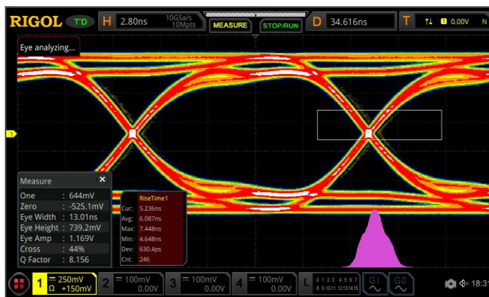
Figure 13: Eye Diagram with improved noise.
