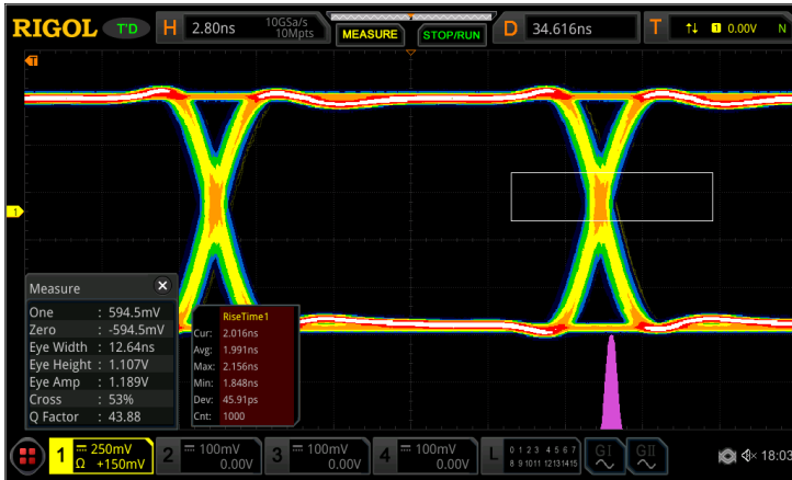
Figure 14: Eye Diagram after debugging and improvements.
