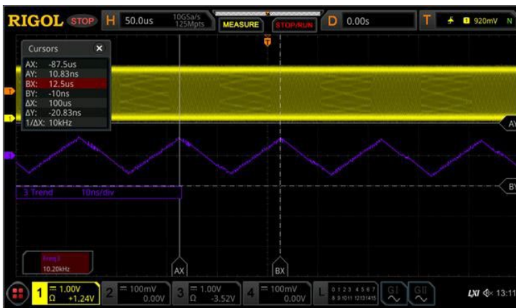
Figure 3: TIE trend graph cursor measurements
