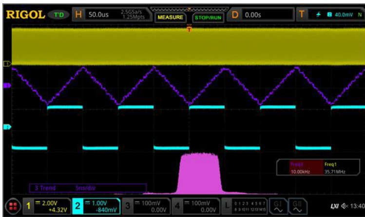
Figure 5: Finding root cause with jitter analysis.
