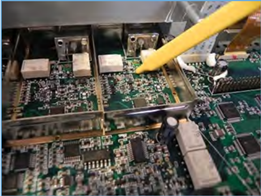
Figure 7-10: Using a near-field probe on an unshielded oscilloscope analog input circuit.
