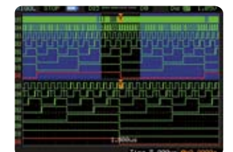
Duration Trigger A combination of Pattern Trigger and Pulse Width Trigger capabilities make isolation of events easy
