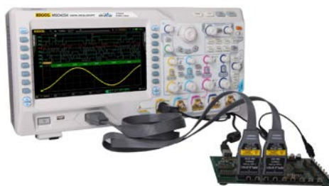
Figure 10 To Connect the Logic Probe
