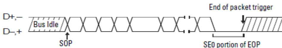
Figure 5-8 USB Data Transmission Protocol
