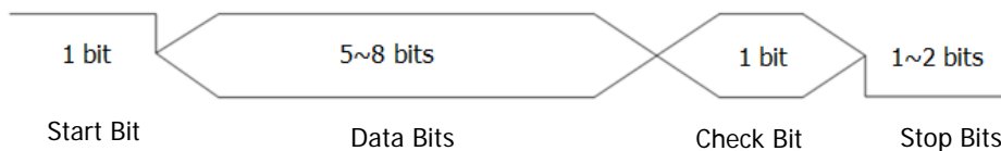
Figure 5-2 RS232 Bus Frame Format
