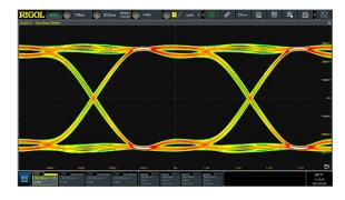
The jitter analysis is mainly used to measure and analyze the clock jitter. The DS70000 series can accomplish the following jitter analysis items.Among the items,TIE is the most commonly used jitter specification.
