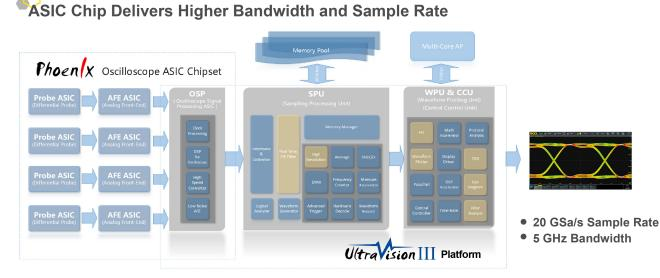
DS70000 series digital oscilloscope is equipped with "Phoenix" chip set, which delivers a max. of **20 GSa/s sample rate** and **5 GHz bandwidth** to better achieve signal fidelity, cover more application scenarios, and cater to the diversified application demands of the complex test system in the industry and R&D fields.
