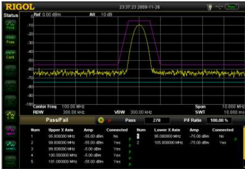
Figure 2-23 Interface of Pass/Fail measurement
