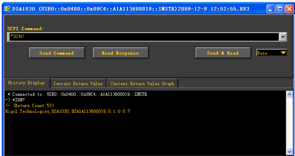
Figure 4-3 Write and read commands via USB
