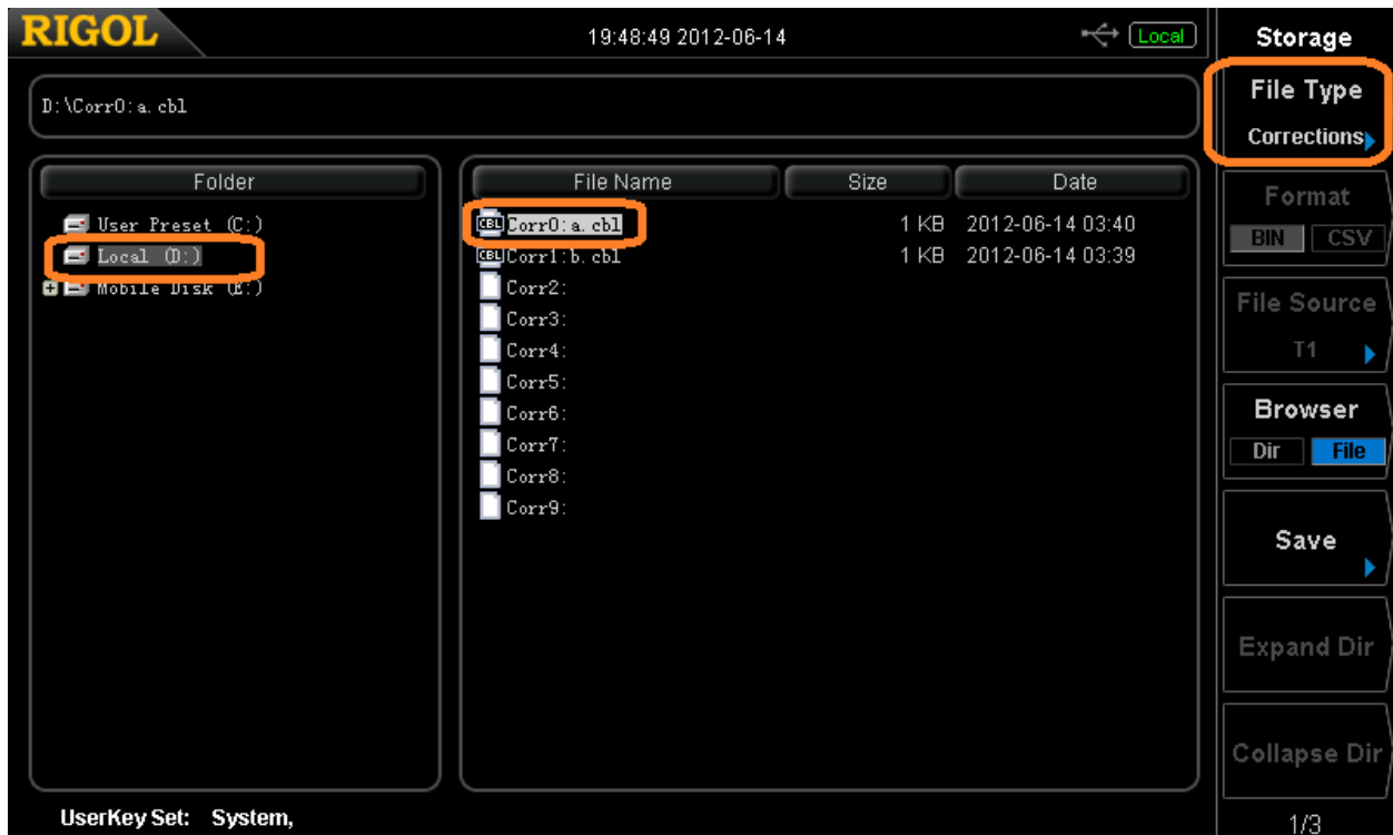
Figure 2: Storage screen for the DSA. Note the Local drive is selected (Left hand side) as is the first corrections file shown. The filter type is set to Corrections. Correction files terminate in *.cbl.
