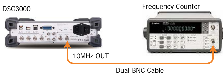
Figure 2-1 10 MHz Reference Output Accuracy Test Connection Diagram
