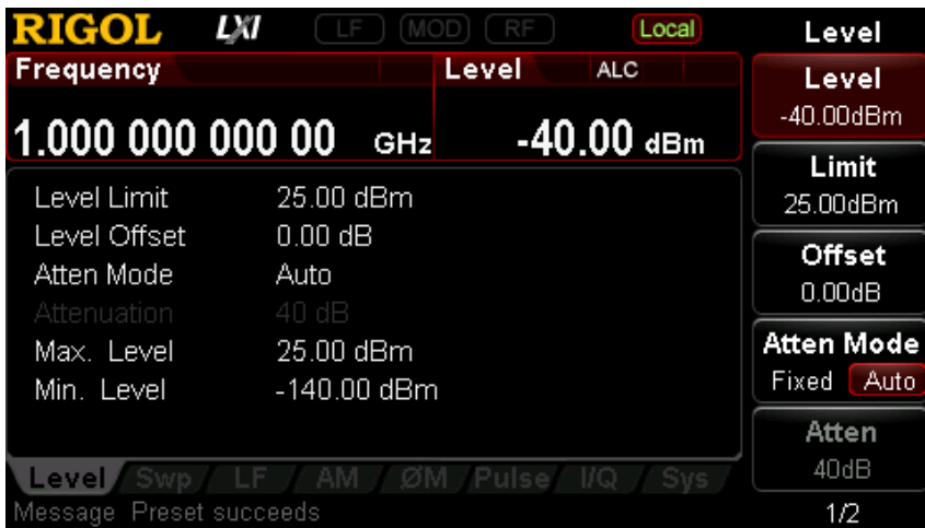
Figure 9 Parameter Setting Interface (To Output RF Signal)
