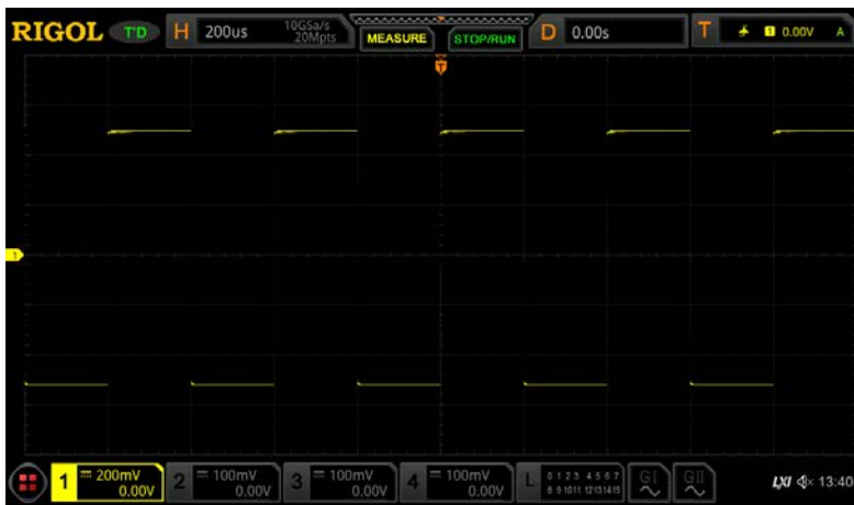
Figure 4-3 Waveforms after 128 Times of Averaging
