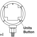
4. Select unit of temperature by using the tip of a pencil to press the units button on the back of the gauge for two seconds until the temperature indicator on the LCD begins to flash. The gauge is now in temperature unit selection mode.
