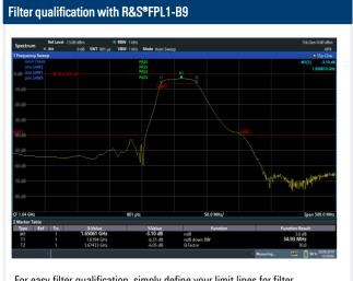
For easy filter qualification, simply define your limit lines for filter characterization, use the n-dB down function to determine the 3 dB points and save the result as a transducer factor
