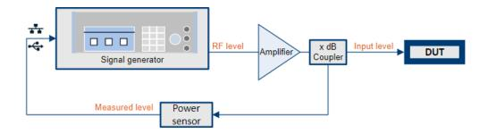
When enabling power control, a control loop is established to stabilize the RF power at a specific point in the measurement setup. The generator continuously or on demand queries the selected power sensor and adjusts
