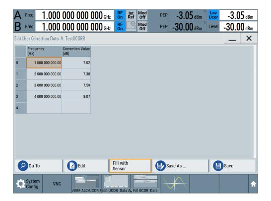
Part of this editor is a feature to fill the level correction points by means of a power sensor. Instead of evaluating and entering each single point, the correction values for a predefined list of frequencies can be determined by a power sensor in a single operation.
