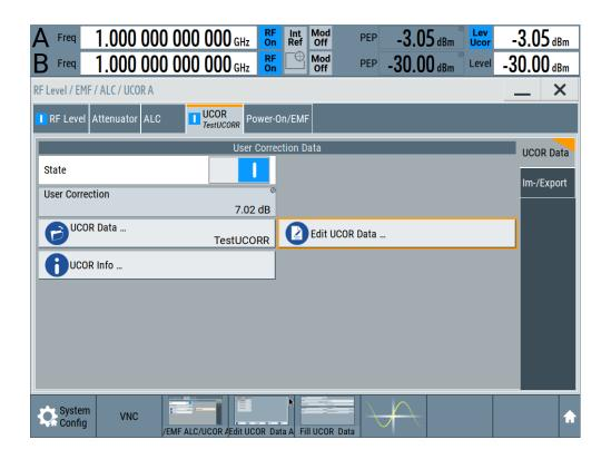
The generators provide an editor to create and modify user correction tables by filling them with a list of frequency- and corresponding level correction values.
