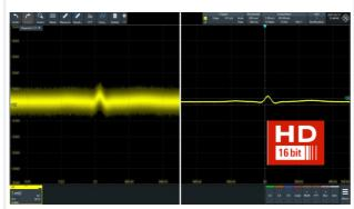
The unique digital trigger system from Rohde & Schwarz uses the sampling points of the A/D converter in the acquisition path so that the trigger system's input data is identical to the displayed signal. The trigger system runs in HD mode with up to 16-bit vertical resolution. This results in a very high trigger sensitivity. You can reliably isolate even the smallest signal details.
