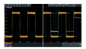
R&S®RT06 oscilloscopes acquire and display up to 1 million waveforms/s in real-time. To make this possible, Rohde & Schwarz developed an ASIC with optimized signal processing. R&S®RT06 oscilloscopes enable you to quickly and reliably detect sporadic signal faults. A high acquisition rate is even available when histograms, masks or cursor measurements are active.
