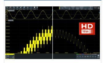
The low-noise frontend and 10 GHz single-core A/D converter are the foundation for the extraordinarily high measurement accuracy and dynamic range of the R&S®RT06 oscilloscopes. The high definition mode (HD mode) activates a configurable hardware lowpass filter, increasing the vertical resolution to up to 16 bit and 9.4 ENOB. Since filtering reduces quantizing noise, signal details become visible.
