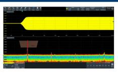
R&S®RT06 provides multichannel FFTs that enable spectrum analysis on every channel with individual settings (center frequency, frequency span, resolution bandwidth) and > 1 000 000 waveforms/s update rate. Overlapping FFT and zone trigger in frequency domain help to identify challenging EMI problems: Detecting and analyzing sporadic emissions.
