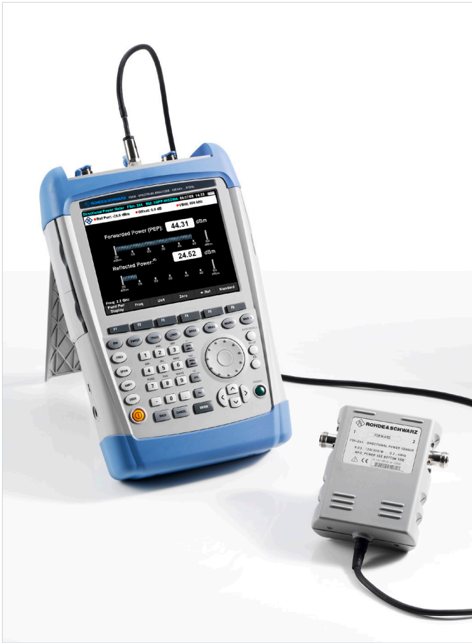
The R&S®FSH and the R&S®FSH-Z44 directional power sensor
