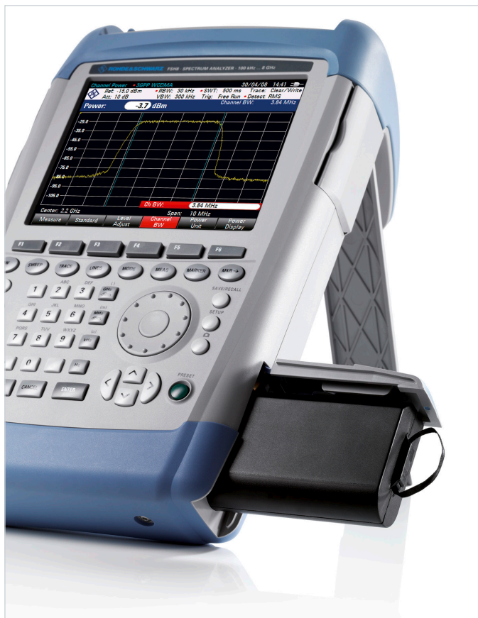
Easy-to-replace lithium ion battery for up to 4.5 h of operation
