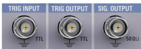
Fig. 7.1: Outputs on the front panel
