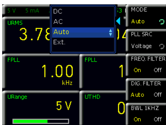
Fig. 6.28: Selecting the data acquisition mode.
