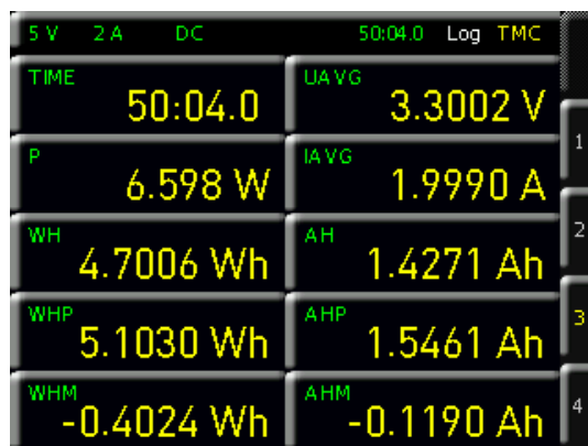
Fig. 6.23: Readout display with integrator output values.
