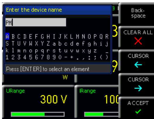
Fig. 9.4: Entering the instrument name.
