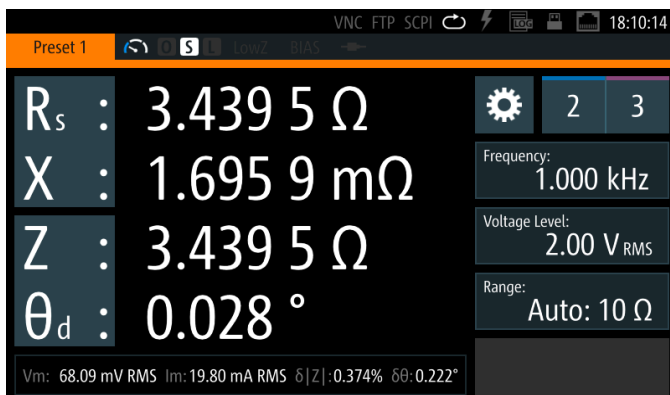
Up to four measurement parameters can be shown on the display at the same time
