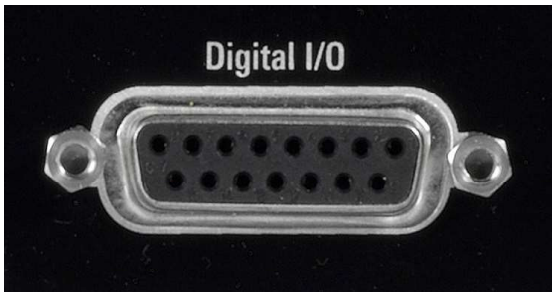
Digital I/O ports on rear panel
