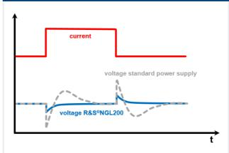
During challenging load conditions, most power supplies react with slow recovery times and overshoots. Specially developed circuits in the R&S\*NGL200 series achieve a load recovery time of  $<30~\mu s$  with minimal overshoot, making them perfect for supplying sensitive components
