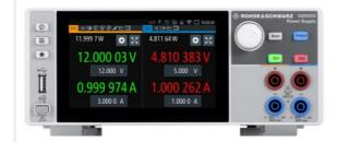
When the power supply is in constant voltage mode, the numbers and the keys are green. Red is used for constant current mode. The output key lights up blue to indicate that the channels are switched on (active).
