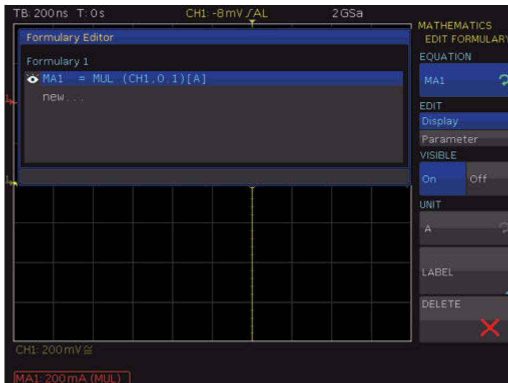
Figure 6-10: Definition of the current equation
