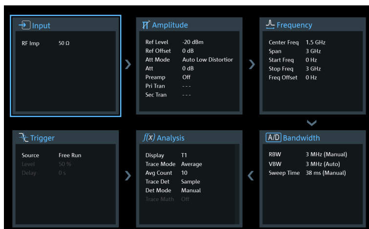
Figure 15-1: Configuration overview in the spectrum application
