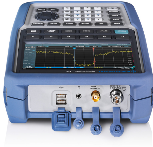
Protected connectors and interfaces
