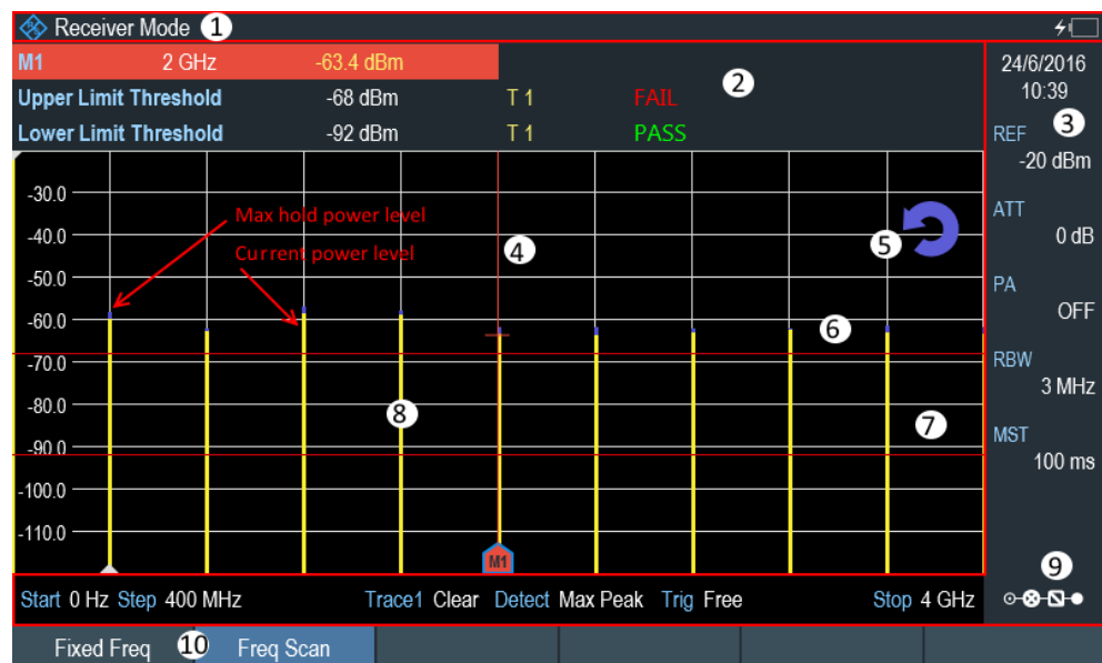
Figure 12-1: Frequency scan measurement
