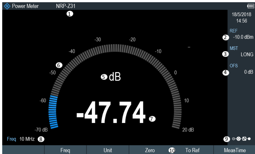
Figure 7-1: Screen layout of the power meter mode
